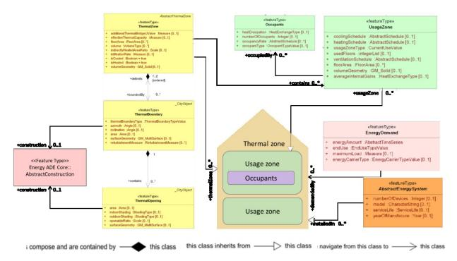
Figure 10: Principal Energy ADE modules interaction in a building core following CityGML format
