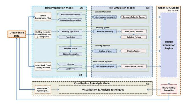
Figure 5: Structure and data flow of the urban building energy system [13]
