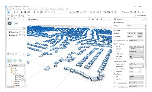
Figure 40: The generated 3D city model using ArcGIS CityEngine and "Building\_From\_Footprint.cga" predefined ruleset to model the buildings in LOD2 using the eave height, ridge height (maximum building height), and roof type attributes alongside the imported footprint
