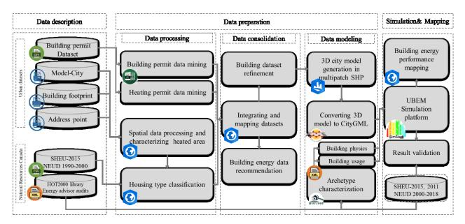
Figure 18: The workflow of urban building energy data preparation, modeling, and mapping using urban datasets
