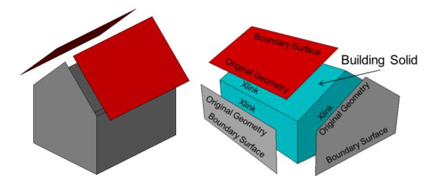
Figure 42: (left) LOD2Multisurface vs. (right)LOD2Solid
