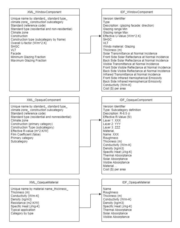
Figure 14: The available information in the opaque components, window (transparent)components, and opaque materials in the XML and IDF versions of elements. It is essential to keep the association between the XML with one of the text formats of IDF, OSM, or OSC.
