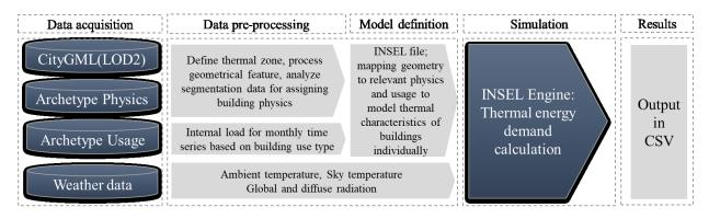
Figure 47: The UBEM data processing using INSEL engine
