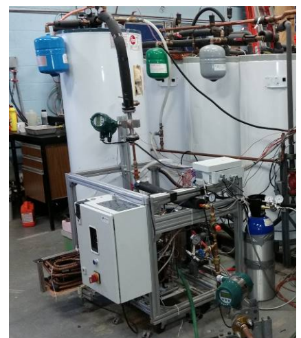
Figure 6. Prototype trans-critical \text{CO}_2 heat pump under test at Queen’s.
