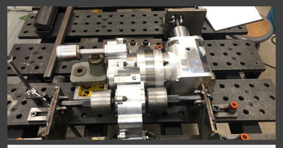
SAE Baja's 4wd drivetrain for internal extracurricular group. A full-scale assembly intended to prepare the next generation of SAE Baja for four-wheel drive.
