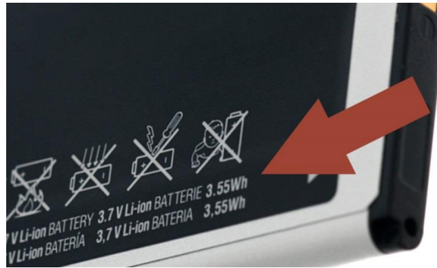
Figure 12: Watt-hour (Wh) rating indications on Li-ion battery
