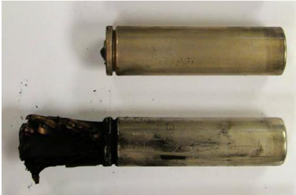
Figure 10: Li-ion cells after thermal runaway: the top cell did not eject its contents (SOC = 0); the bottom cell did (SOC = 100%)
