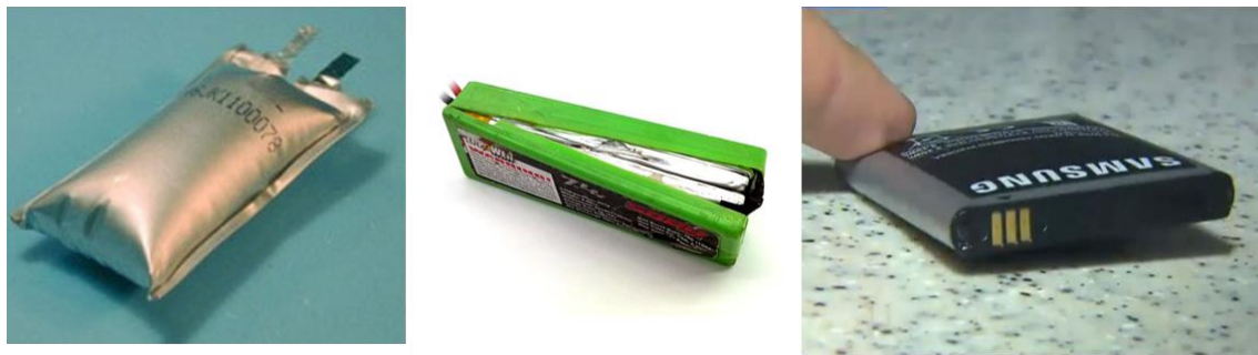
Figure 7: Swollen lithium batteries
