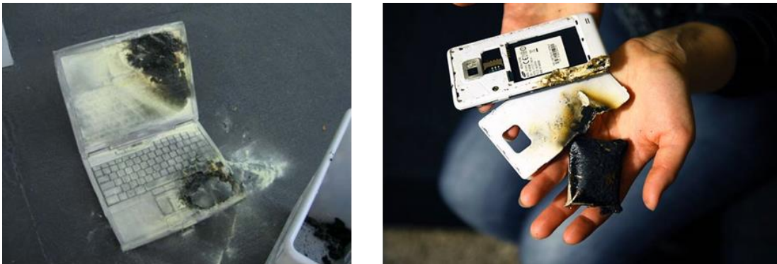
Figure 8: Results of lithium battery fires
