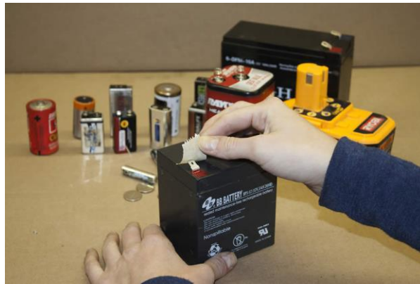
Figure 14: Protecting battery terminals
