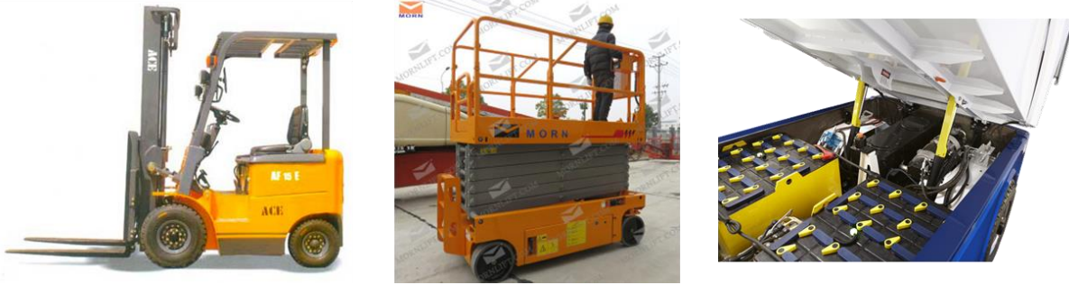
Figure 9: Examples of vented lead acid powered equipment or vehicles; from left to right: forklift, scissor lift and ice resurfacer
