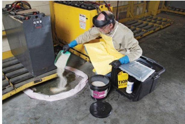
Figure 3: Picking up a small battery electrolyte spill
