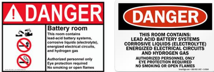
Figure 5: Examples of lead-acid battery danger signs (ANSI and OSHA respectively)
