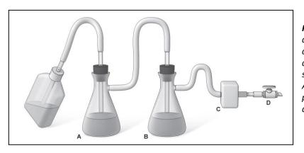
**Figure 1**: Flask (A) collects the contaminated fluids into a suitable decontamination solution; flask (B) also contains a suitable decontaminant and serves as a fluid overflow collection vessel. An in-line HEPA or 0.2 μm filter (C) protects the vacuum system (D) from aerosolized microorganisms or toxins.
