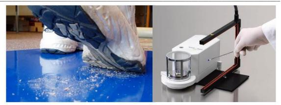
Figure 20: Example of tacky mats and laboratory anti-static devices
