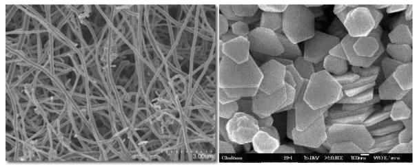
Figure 2: Carbon nanofibers (left) and silver nanoplatelets (right)
