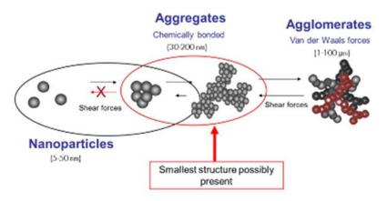
Figure 3: Nanoparticle aggregates and agglomerates
