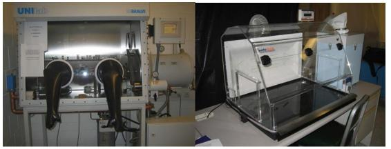
Figure 19: Examples of enclosed systems
