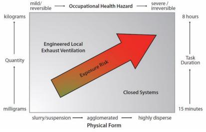
Figure 17: Engineering controls vs exposure risk to nanoparticles
