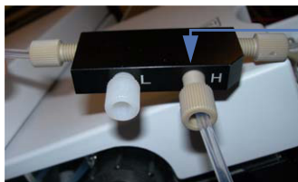
Figure 3 Dual AJS ESI source plumbed for low flow application. The “H” indicates high restriction of gas flow.
